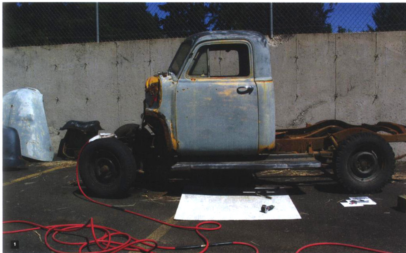
1 As with any project, the disassembly and inspection of the new project truck was the first order of business for the Chevs of the 40's crew. The truck was in very solid condition with little rust. A great find, by the way.
